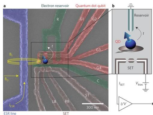
**Figure 4 - False-coloured SEM image (a) and schematic diagram (b) of a Si quantum-computing device**
